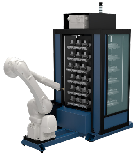
EZ-TEND™ Non-intimidating industrial robotic machine tending platform
